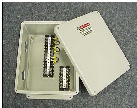
10 x 8 x 6" NEMA 4X, fiberglass example shown with pre-jumpered, 600 vac rated Marathon terminal blocks. This size and design of PJB enclosure is typically used on systems that involve twelve or fewer heating modules per hopper.
